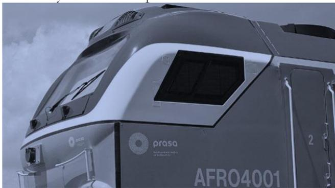
The new locomotives were designed in Spain by rail industry manufacturer Vossloh according to Prasa specifications to suit local conditions and come fitted with the latest technology. They have a driver display unit with route and train management systems for the driver to detect and reset any faults. It is the first diesel locomotive in the country to have two driving cabs; it can be driven both directions without turning.
